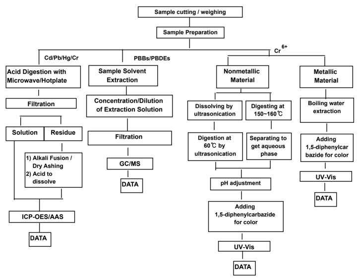
The samples were dissolved totally at the acid digestion step of the above flow chart for Cd,Pb,Hg Section Chief : Sharpless Park
